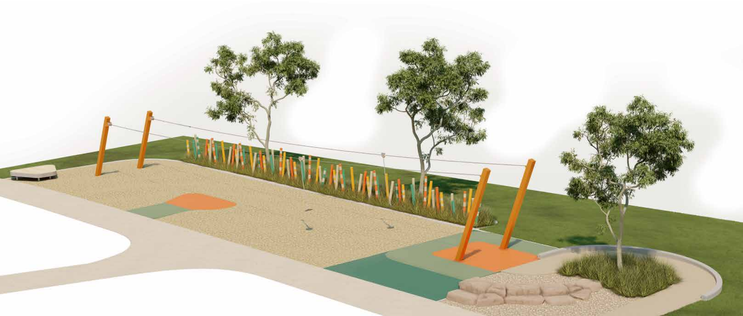
35 Dual Flying Fox with standard pommel seat and an all abilities bucket seat. DDA compliant access to top of 'take off' mound.
